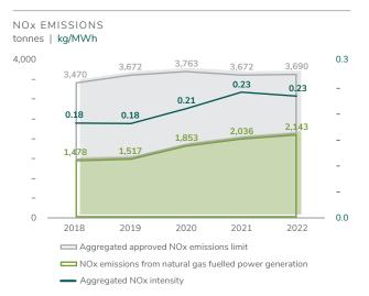
We maintain NOx emissions levels from our operated power generation facilities below our allowable NOx levels. However, to reduce excessive wear on equipment, we have had to reduce ammonia injection (one of our NOx reduction methods) and, therefore, have seen an increase in absolute and intensity NOx emissions levels when compared to previous years.
