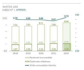
Our water intensity increased over the last year due to the high utilization rates of our natural gas-fueled generation facilities. Most of the water we use is non-potable and for power generation cooling processes.
