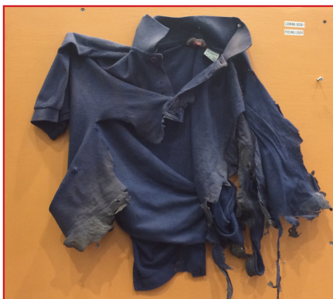
Remains of a shirt worn by a worker after an electrical arc flash incident.
